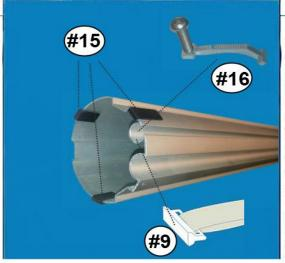
Evenly space three #15 tube clips around end (without drilled hole) of each Inner tube D. Slide the inner tube D into outer tube E and adjust the width to suit the pool. Insert locking pin #16 into the keyway on each inner tube D. Slide one #15 clip over outer tube opposite locking pin. Insert #9 strap connectors into the tube keyway on all tubes and space evenly between 600mm and 900mm apart.
